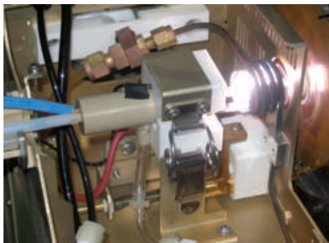
The UMAS ion source installed in a conventional ICP-MS system
